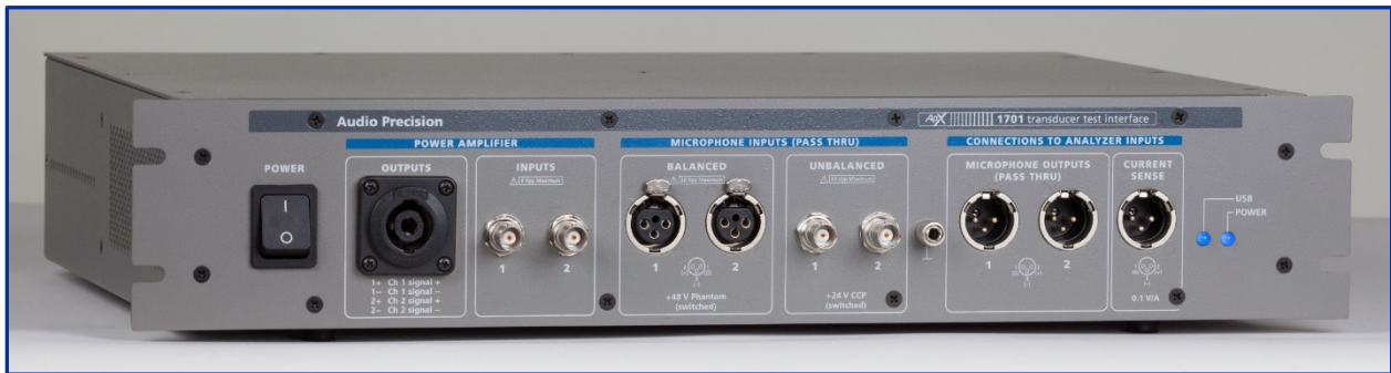
Figure 18. The APx1701 Transducer Test Interface.
